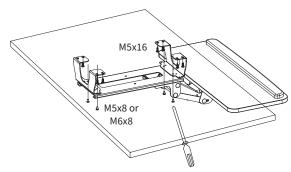
Attach brackets to ends of VIVO under desk keyboard tray using M5x8 or M6x8 screws. Mark drilling locations under desk with a pencil, drill pilot holes with a 3/32" drill bit, and mount keyboard tray with brackets to desk using M5x16 screws.
